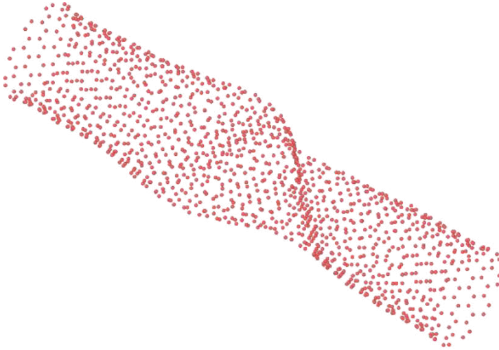
Figure 4. Shell-like buckling failure of a SWCNT(10,10).
