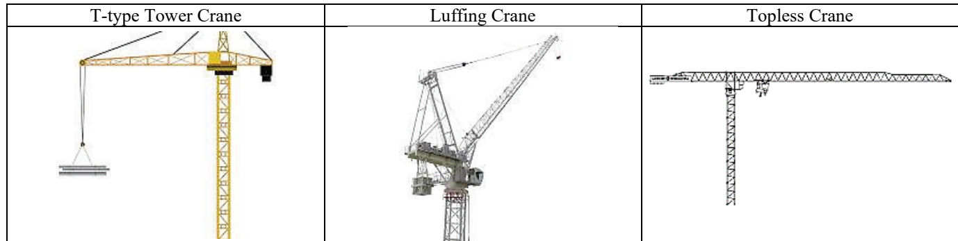
Figure 1 "T-type" and "L-type tower crane", Topless crane
