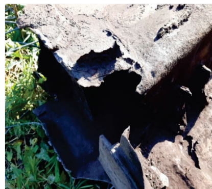
Figure 2 Breakage of the side panel from the fastening points
