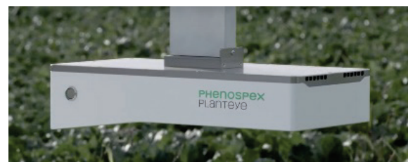
Figure 5 Laser Scanner PlanTeye builds 3D point clouds [34]
