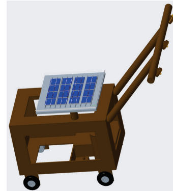
Figure 9 3D CAD model of the chassis
