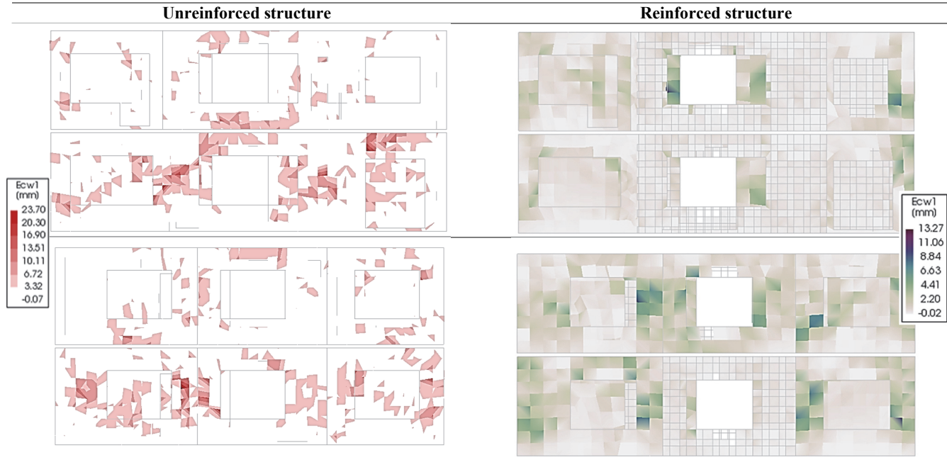
Figure 30 Distribution of and crack width
