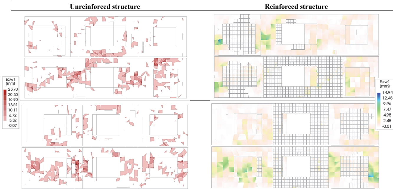
Figure 27 Distribution of the crack widths
