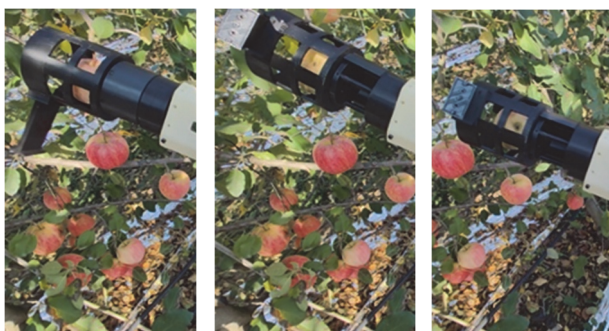
Figure 9 Actual harvesting process of the end effector
