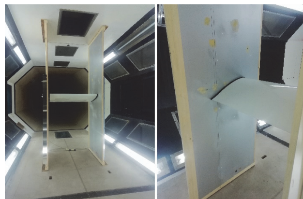
Figure 11 The NA-DEL 2415 airfoil model used in wind tunnel experiments, mounted between boundary plates
