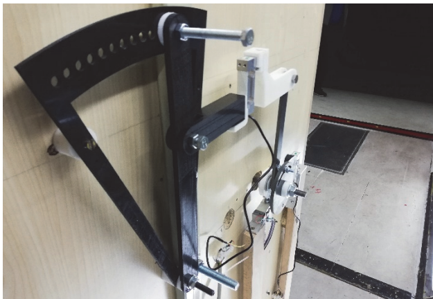
Figure 8 The real-life manual system for AoA settings
