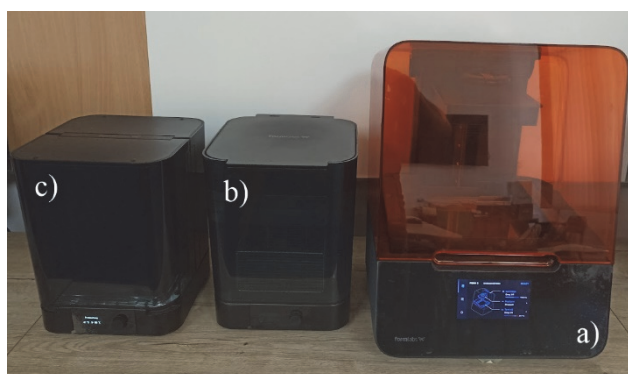
Figure 3 Formlabs form 3 setup: a) Form 3 printer; b) Form wash and c) Form cure
