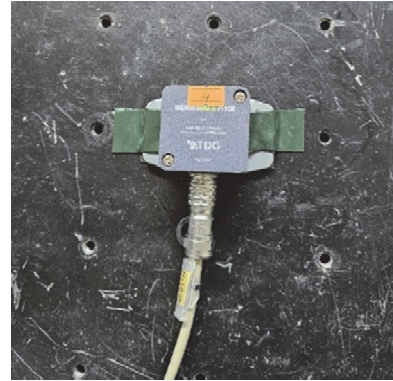
Figure 3 Sensebox 7001 accelerometer attached to the shaking table
