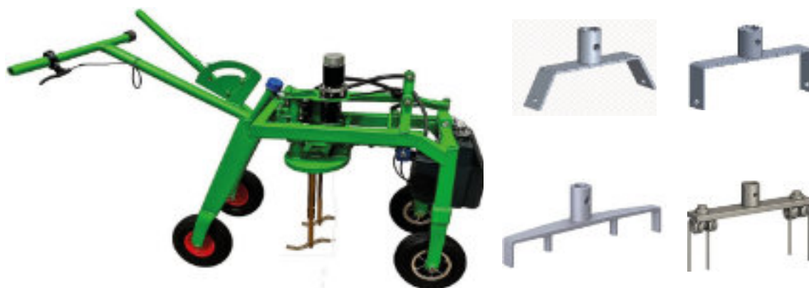
Figure 1. 3D model of the hoeing robot and its different hoeing elements
