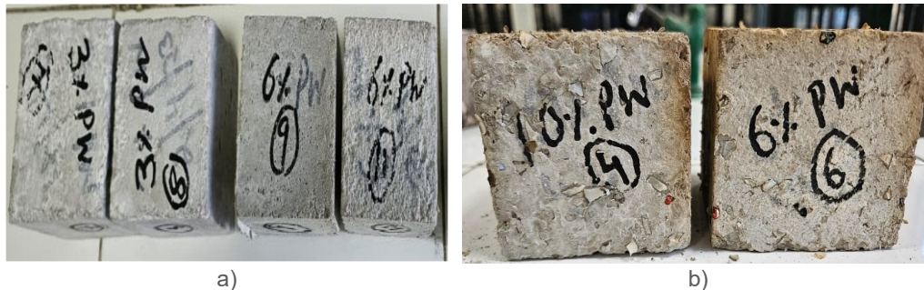
Figure 3. Mortar mix containing plastic: a) before exposure to high temperature, and b) after exposure
