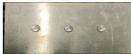
Fig. 14 Riveting structural parts
