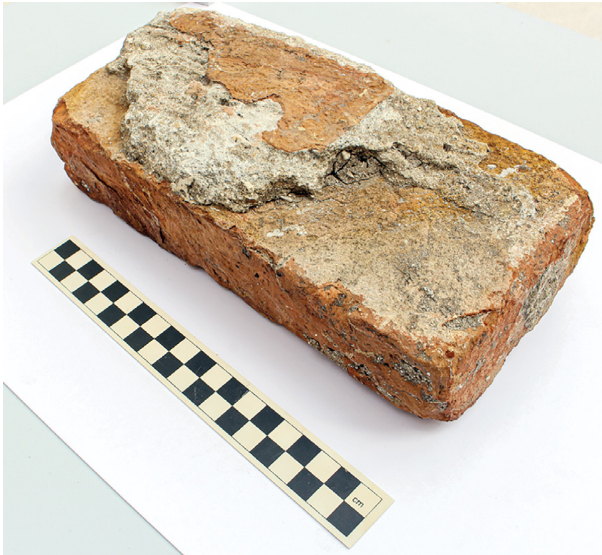
SLIKA 10. Opeka s ostatkom žbuke (snimio: R. Surić) FIGURE 10 Brick with mortar adhering (photo by R. Surić)
