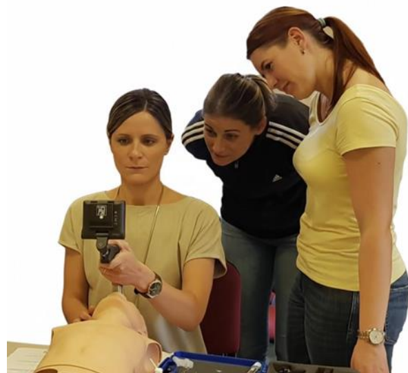
Figure 3. A training of endotracheal intubation on a mannequin using a video laryngoscope. A small video monitor is attached to the laryngoscope handle, displaying a magnified view from a camera located near the tip of the blade, allowing a shared view and realistic medical training on a simulator.
