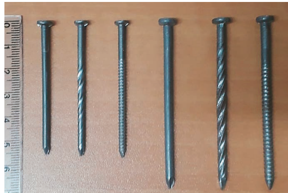
Figure 1 Nails used in withdrawal tests: smooth, helical, and annular with 2.8 mm and 3.5 mm of diameter, respectively
