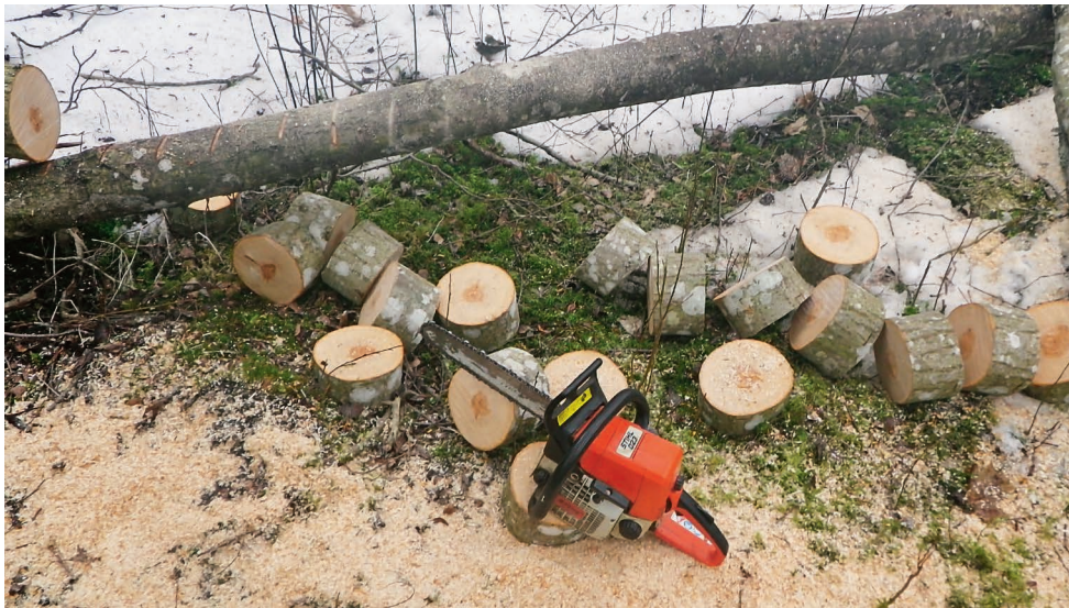
Figure 1 Grey alder stem cut into 10 cm thick discs with 1.9 kW Stihl 023 Slika 1. Deblo drva bijele johe raspiljeno na diskove debljine 10 cm pilom Stihl 023 snage 1,9 kW
