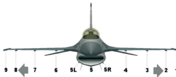
Fig. 1 Underwing store configurations of F-16 fighter jet
