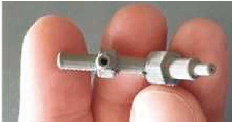
Fig. 7 A usable 3D-printed fuel injector
