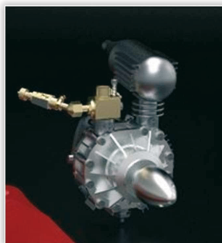
Fig. 2 A 3D model of the Wankel engine visualised in the software for 3D modelling
