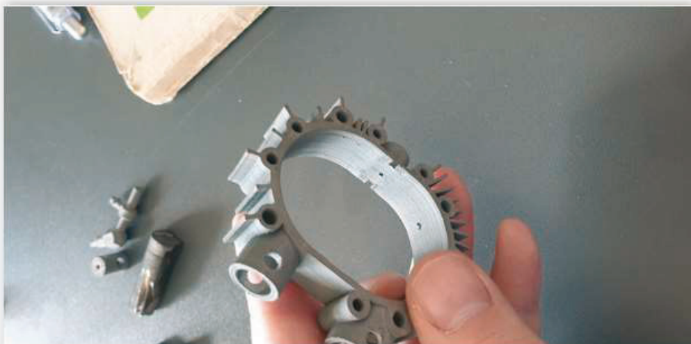
Fig. 9 The housing of the Wankel engine
