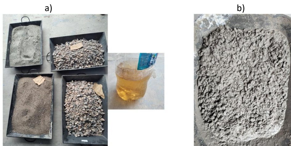
Figure 2. a) Materials to produce concrete: gravel, sand, water, inhibitor and cement; b) concrete paste
