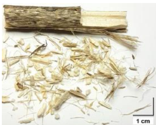
Fig.3 The depiction of Virginia mallow stem before and after grinding by the hammer mill [26]
