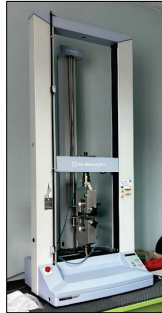
Figure 2 Shimadzu AGS-X tensile testing machine
