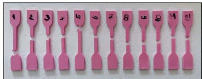
Figure 4 Test samples without an adhesion layer after the tensile strength test
