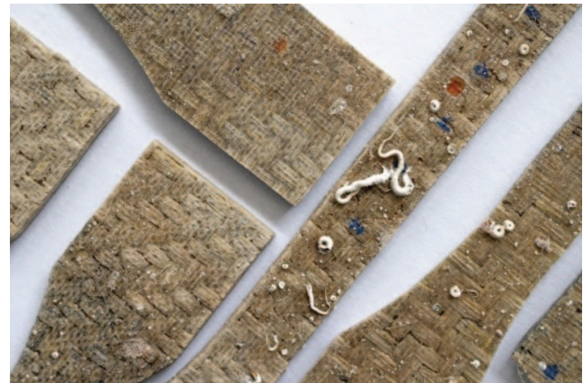
Figure 9 Close-up of bio growth accumulation.
