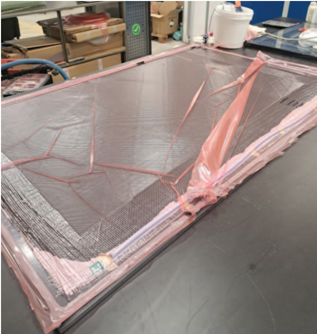
Figure 4 Vacuum infusion process
