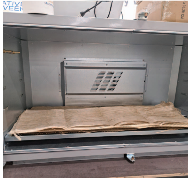
Figure 1 Material dehumidification in the curing oven
