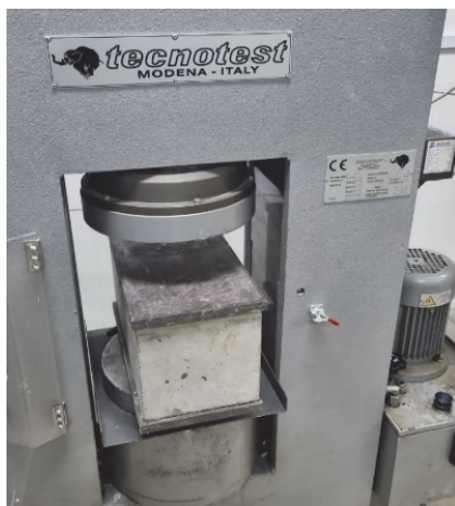
Figure 7 Hydraulic press used in the compression strength tests
