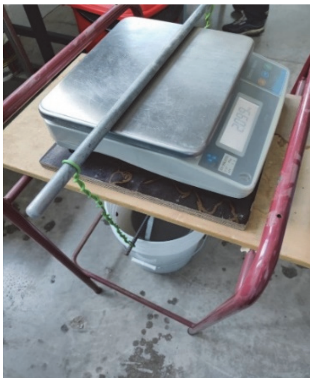
Figure 10 Water absorption test with the block submerged
