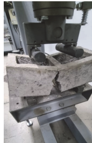
Figure 8. Hydraulic press used in the flexural-tensile strength tests
