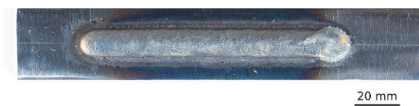
Figure 8 Bead appearance, ALC 0, DC 10
