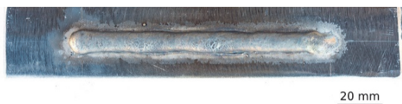
Figure 3 Bead appearance, ALC -10, DC 0
