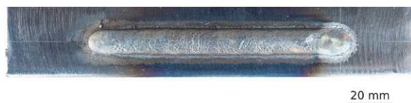
Figure 4 Bead appearance, ALC 0, DC -10
