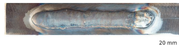
Figure 7 Bead appearance, ALC 10, DC 0
