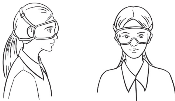
Figure 10 Design of redesigned goggles for stretcher bearers
