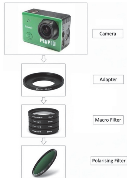
Figure 2 Camera modification diagram
