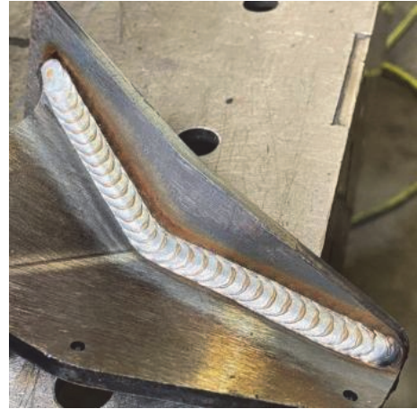
Figure 6 Weld seam type III
