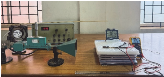
Figure 21 Photograph of experimental set-up for powering the sensor using the proposed rectenna
