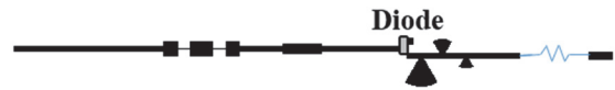
Figure 10 Layout of the rectifier circuit featuring a two section quarter wave transformer, LPF and DC pass filter
