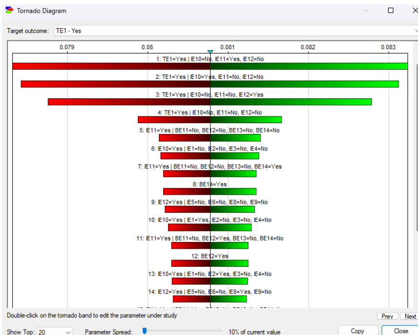
Figure 10. The result of sensitivity tornado with Top Event failure as the target
