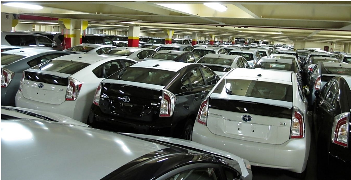
Figure 2. Standard vehicle stowage on board Pure Car Carriers
