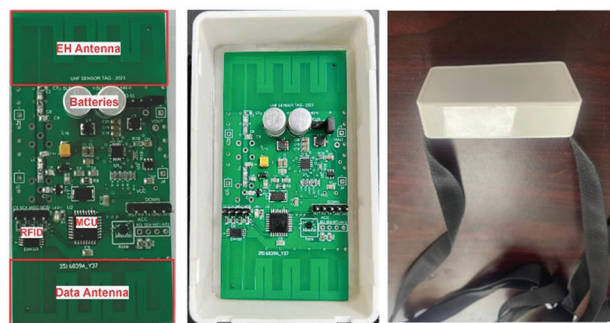
Fig. 2. The proposed sensor tag
