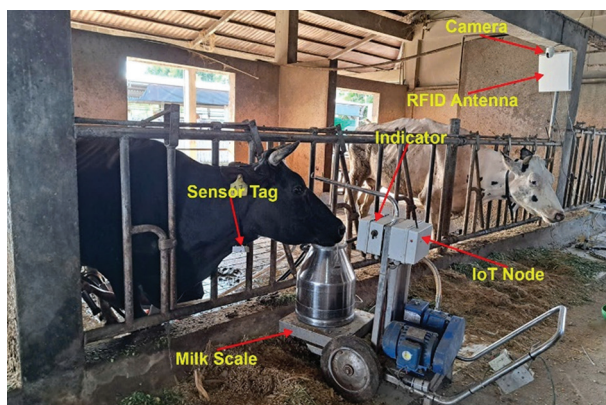
Fig. 6. Experimental setup at the Tan Tai Loc dairy cow farm
