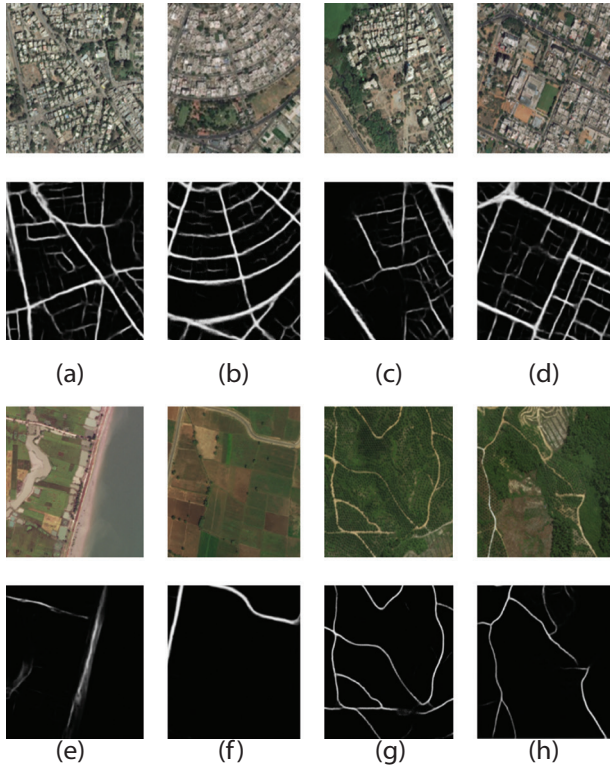
Fig. 5. The results of the proposed model on different images. (a), (b), (c), and (d) represent the satellite images (different urban and residential areas) with the road maps obtained from the proposed model. (e), (f) (g), and (h) represent the satellite images (different agricultural and rural areas) with the road maps obtained from the proposed model
