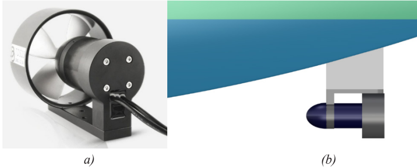
Figure 13. Motor replacement: (a) 6 TDS10 motor, (b) motor placement.
