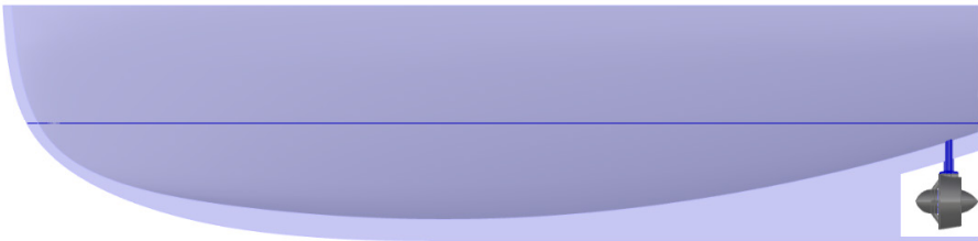
Figure 1. One of abandoned concepts with long straight keel.
