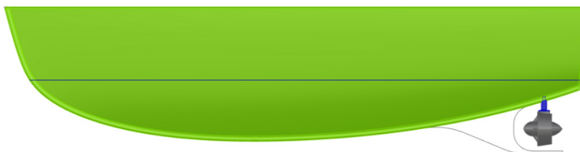
Figure 3. Concept 06a-100, L = 2400 mm, B = 300 mm, D = 300 mm, F = 300 mm.
