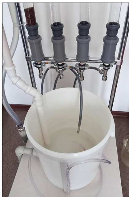
Figure 2. Laboratory setup showing the column apparatus used for TDS leaching experiments.
