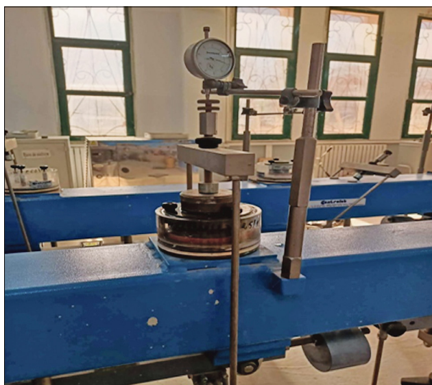
Figure 6. Sample under consolidation
