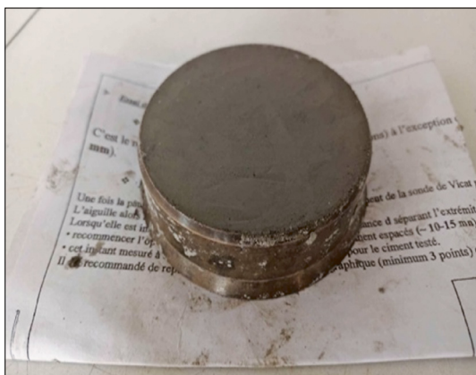
Figure 5. Soil filled in the cylindrical mold
