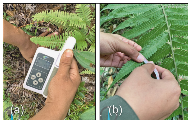
Figure 5. Field documentation of SPAD verification: (a) SPAD measurement on ferns exhibiting stunted growth and pale green colouration; and (b) SPAD measurement on ferns with healthy appearance and greener leaves.
