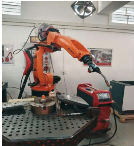
Fig. 1 CMT welding setup with a robotic arm
