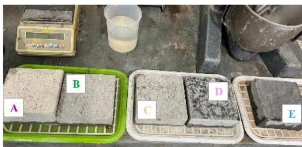
Figure 3. Mortar specimens during capillary water absorption testing
