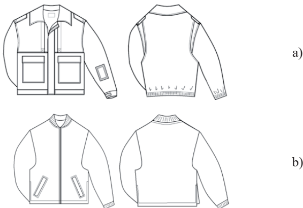
Fig. 3. Model sketch of protective garment system: a) outer shell (IM1+IM2); b) removable thermal insert (TU1: IM3+IM4 and TU2: IM3+IM5)
