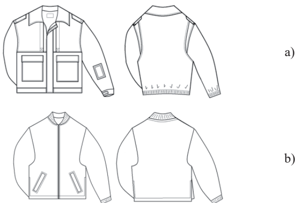
Fig. 3. Model sketch of protective garment system: a) outer shell (IM1+IM2); b) removable thermal insert (TU1: IM3+IM4 and TU2: IM3+IM5)
