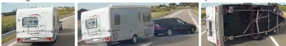
Figure 2. An illustration of a road accident due to the sway motion of a trailer
