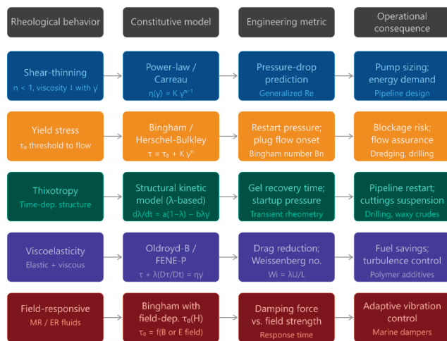
Figure 1 Rheology-to-design-consequence framework adopted in this review. Each row maps a dominant non-Newtonian behavior to its representative constitutive model, the engineering metric it governs, and the resulting operational consequence.
