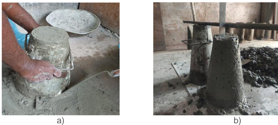
Figure 3. Measuring slump value of the concrete mix: a) filling the slump cone; b) measuring the slump value after lifting the cone
