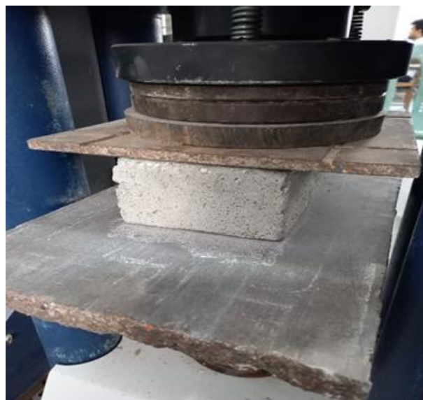
Figure 7. Brick specimen during compressive strength
