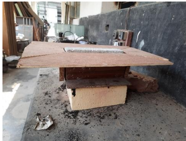
Figure 8. Heat insulation test of brick
