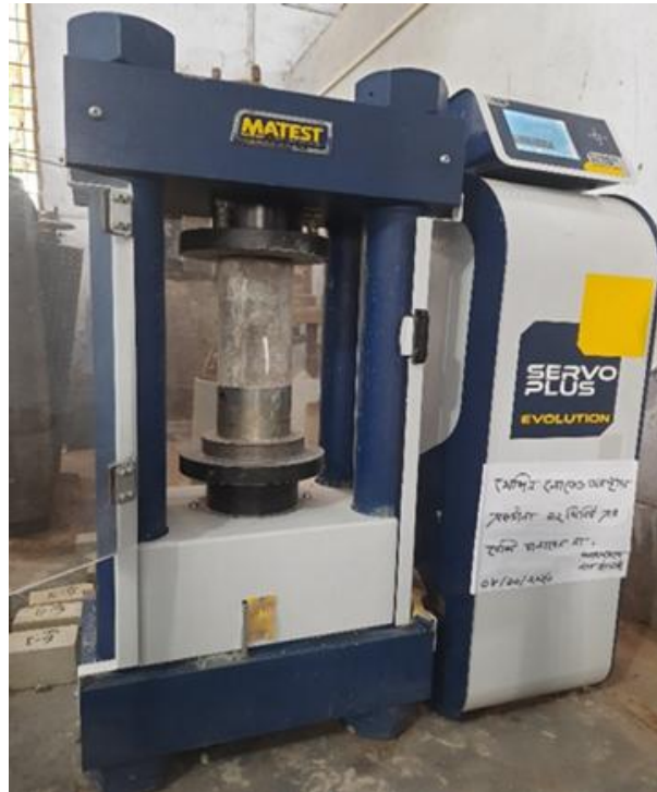
Figure 4. Specimen during compressive strength test
