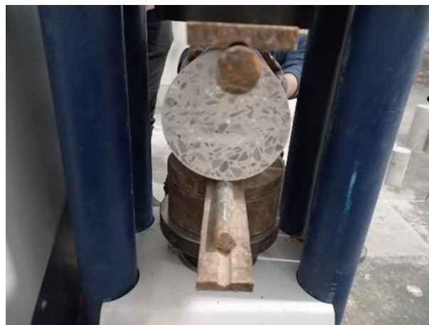
Figure 5. Specimen during split tensile strength test
