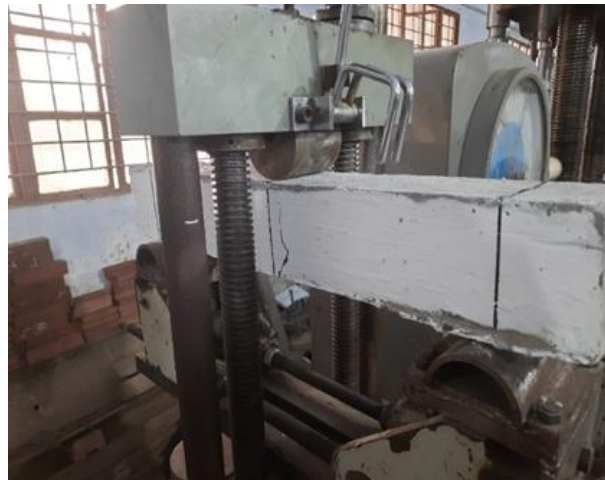
Figure 6. Sample during the flexural strength test
