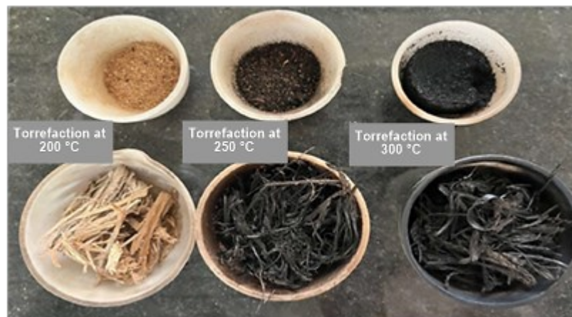
Figure 6. Visual changes in biomass during oxidative torrefaction at 200, 250, and 300 °C
