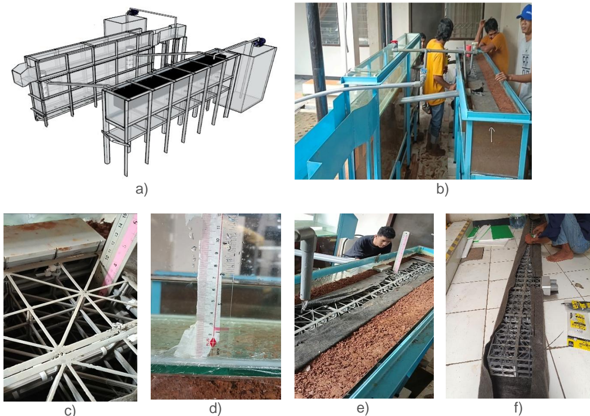
Figure 3. Drainage flume and median flume models: a) three dimensions of flume; b) laboratory flume; c) measurement of water level in infiltration box; d) measurement of water level in drainage flume; e) placement of infiltration box in median flume; and f) assembling the infiltration box into one unit and installing geotextiles
