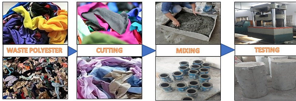
Figure 1. Procedure to use polyester waste fabric for green concrete
