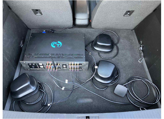
Fig. 3. The image shows the F-Tester ® 4drive-box measurement platform with three 4x4 MIMO multiband measurement antennas and one 2x2 MIMO antenna with an integrated GNSS antenna connected to the orchestration unit. The entire setup is located in the trunk of a car. This placement better reflects the user experience with the mobile network inside the vehicle.
