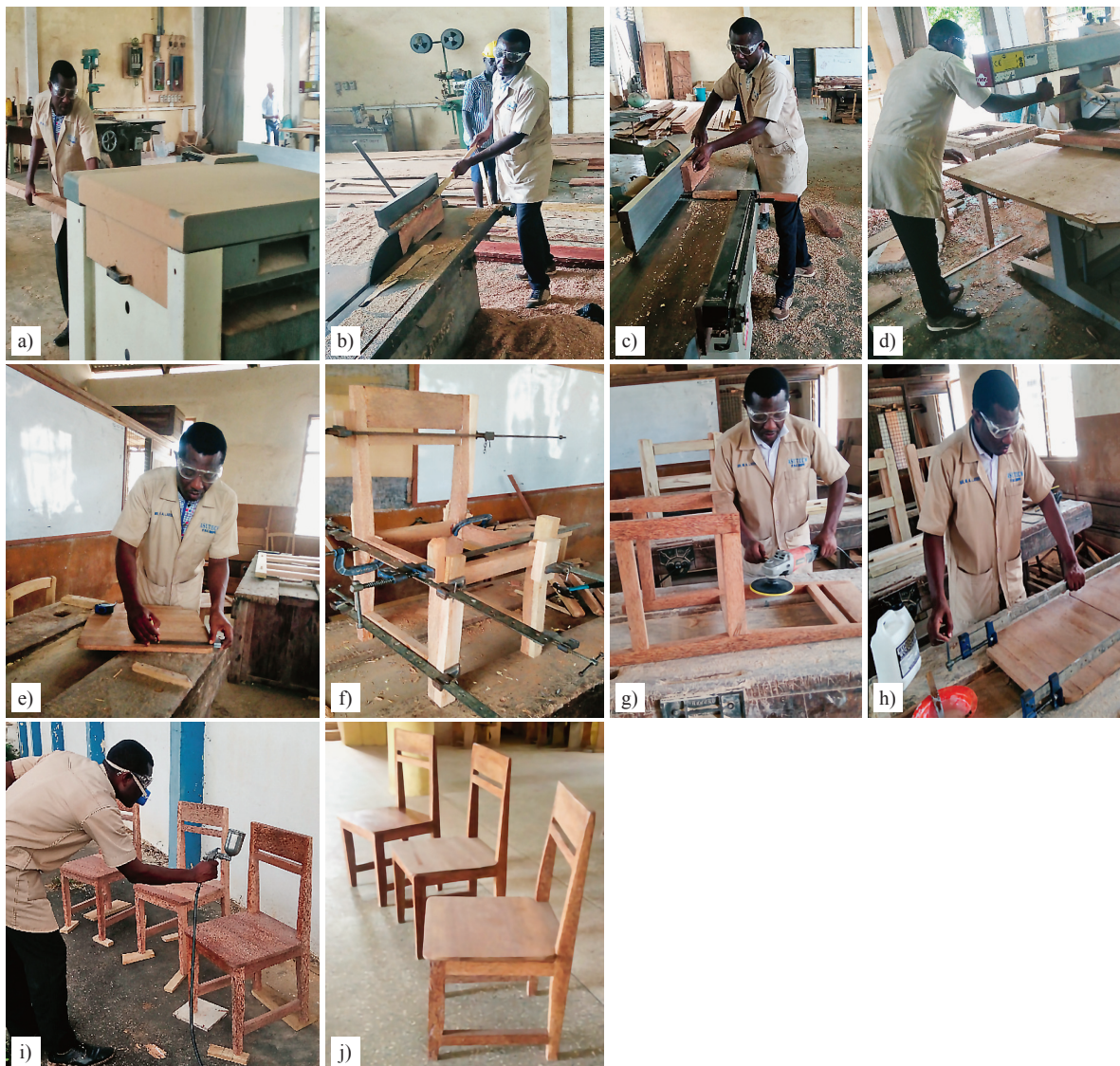
Figure 2 Construction stages of the three coco wood chairs: a) planing, b) ripping, c) shooting, d) cross-cutting, e) marking out and joint construction, f) trial and final assembly of joints, g) sanding of the chair structure, h) lamination of the chair seat, i) application of the final coating material, j) final products
