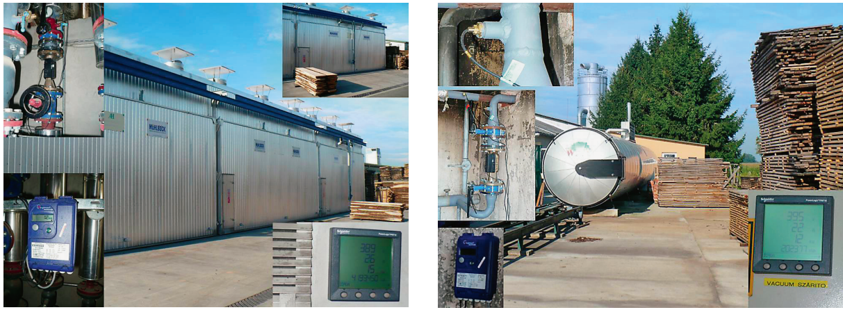
Figure 1 Thermal and electrical energy monitoring and data acquisition setup for convective (left) and vacuum (right) drying systems
