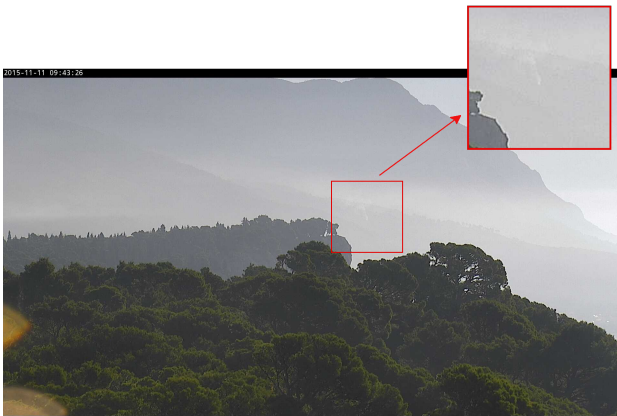
Fig. 5. Original 1920×1080 resolution image taken from a surveillance camera and a positive 224×224 sample containing emerging smoke in its early phase. The smoke sample is shown magnified by a factor of 2.
